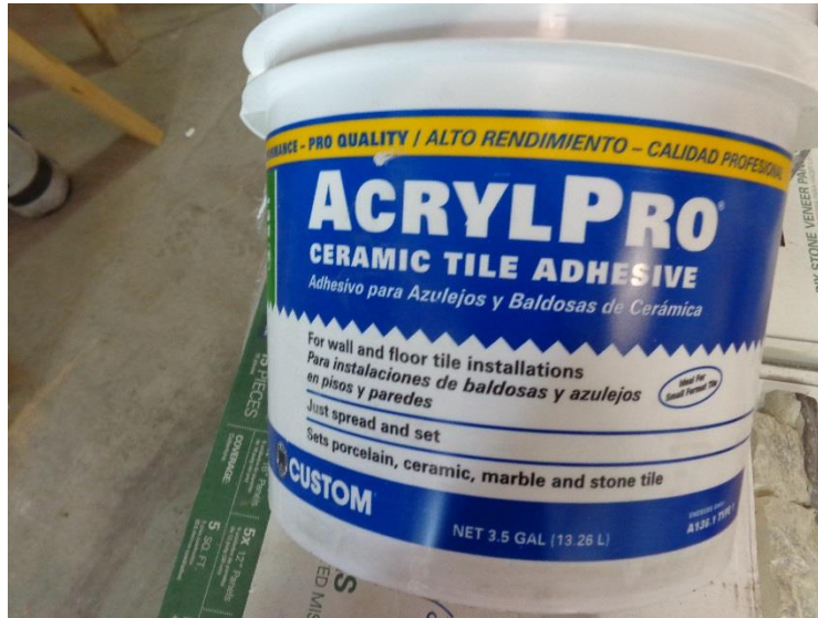
Photo No. 1 Adhesive used to Adhere the Samples
